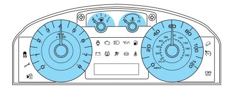
Speedometer: Indicates the current vehicle speed.
